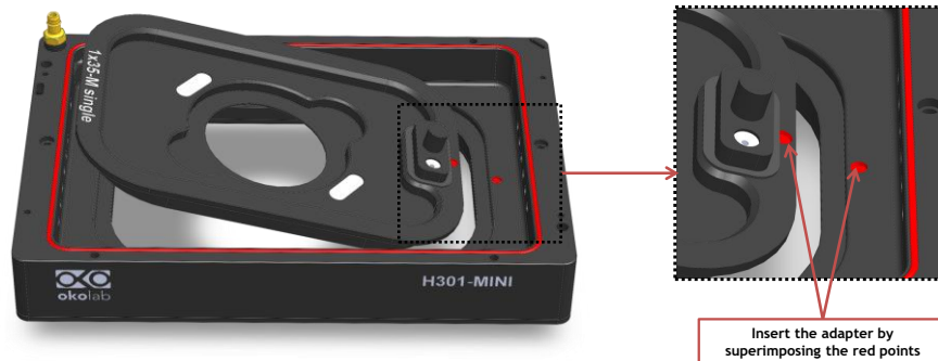
Figure 4. Introduction of the Specimen Holder inside the Chamber Base.
